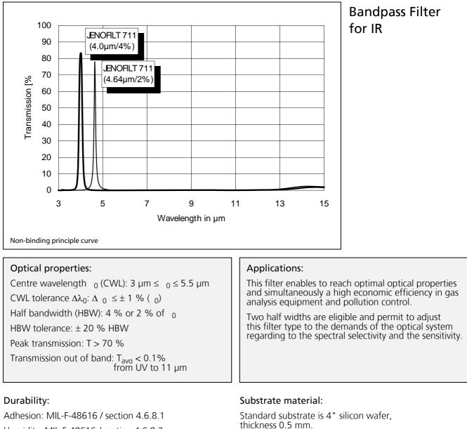
Humidity: MIL-F-48616 / section 4.6.8.2 Abrasion resistance: MIL-F-48616 / section 4.6.8.3
